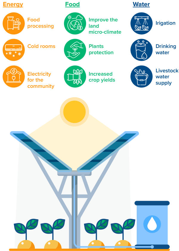
Figure 29. Scheme of agrivoltaics system with triple land use benefits (power generation, food production, and rainwater harvesting). (Source: Fraunhofer ISE, n.d.)
